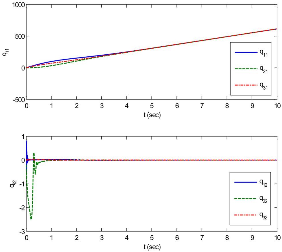
Fig 6. Consensus of joints of the robots
