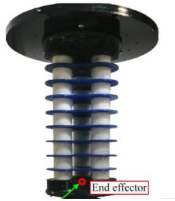
Fig. 4. Soft pneumatic arm; the outcome of each two-stage silicone molding and related 3D-printed mold is presented.
