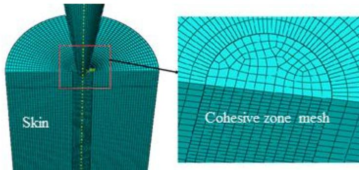
Fig. 3. Mesh of the model in FE.
