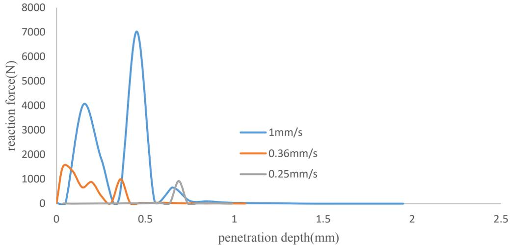
**Fig. 11.** Changes in the reaction force applied to the microneedle by changing the speed (high speeds).
