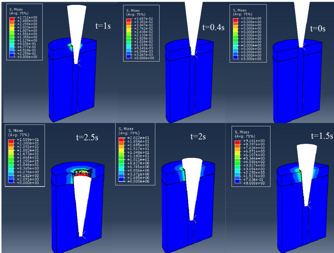
Fig. 7. Stress applied to the skin during the penetration of microneedle.
