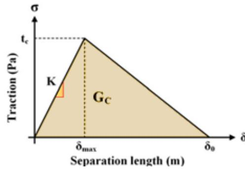
Fig. 2. Traction-separation Diagram [18].
