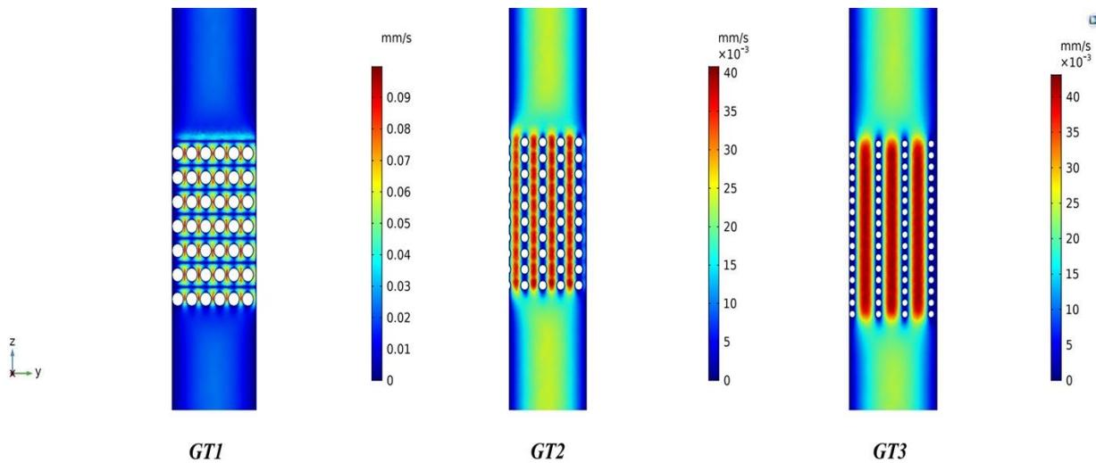
Fig. 5. Velocity magnitude contours within all scaffold architectures. With increasing the porosity, the rate of increased perfusion has been reduced.
