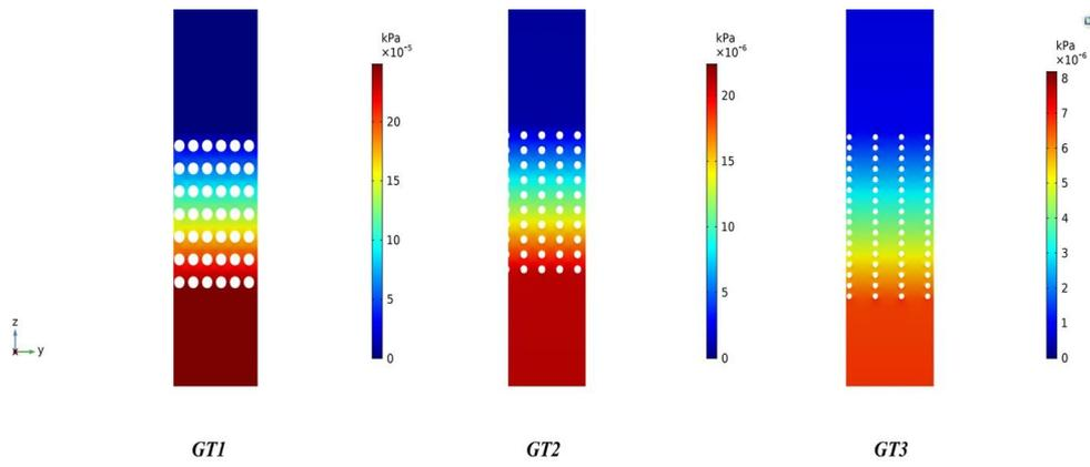
Fig. 7. Pressure distribution contours within all scaffold architectures.
