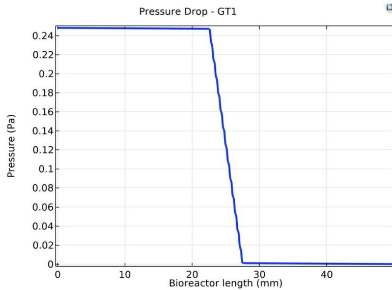
Fig. 8. This diagram depicts the pressure drop of the central section along the bioreactor with the GT1 scaffold. The GT1 scaffold has the highest pressure drop among the designed scaffolds.
