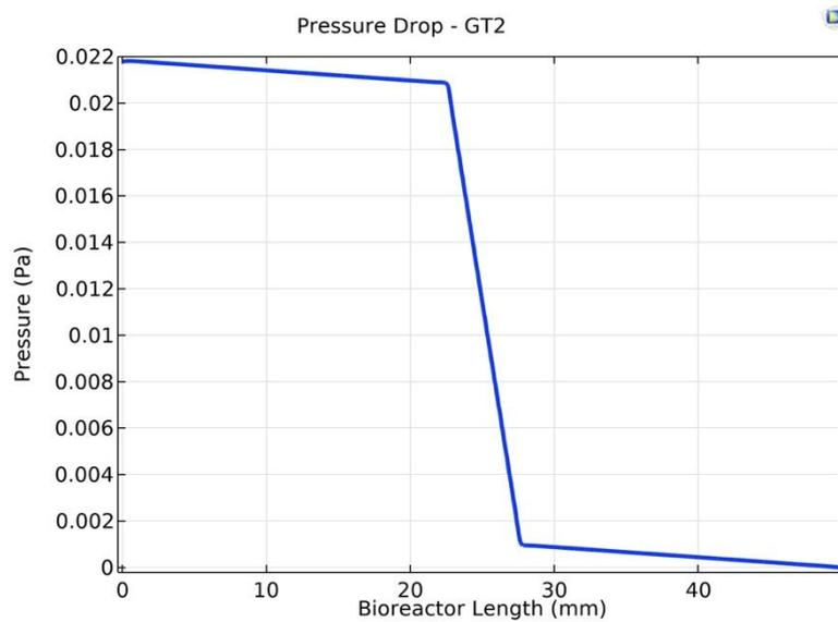
Fig. 9. This diagram depicts the pressure drop of the central section along the bioreactor with the GT2 scaffold.
