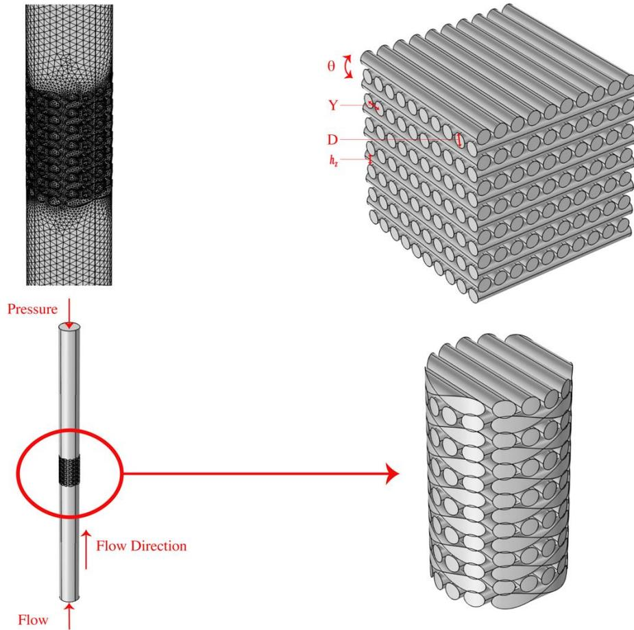
**Fig. 1 . Geometry of the scaffold GT1 with controllable parameters and mesh details.**
