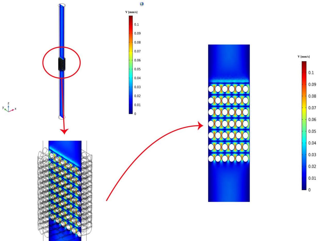
Fig. 3. Velocity magnitude contours within the GT1 scaffold architecture.
