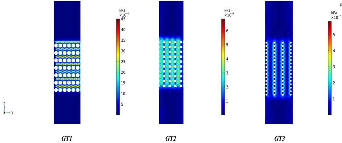
**Fig. 6. Wall shear stress distribution contours within all scaffold architectures. With increasing the porosity, the wall shear stress has been reduced.**
