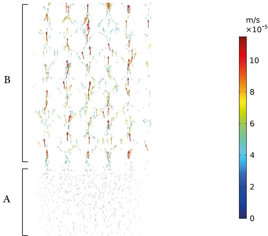
Fig. 4. Velocity field within bioreactor before entering porous domain (A) and inside GT1 scaffold (B) is shown in which an increase in the magnitude of velocity inside the scaffold can be observed.
