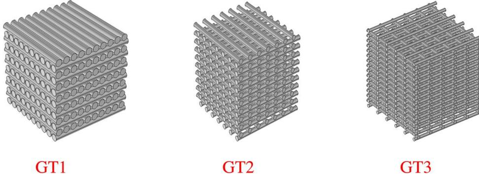
**Fig. 2. Three scaffolds with different porosities. GT1 and GT3 have the least and most porosity, respectively.**
