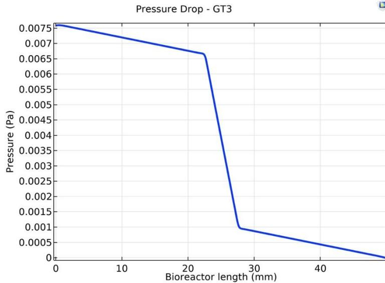
Fig. 10. This diagram depicts the pressure drop of the central section along the bioreactor with the GT3 scaffold.
