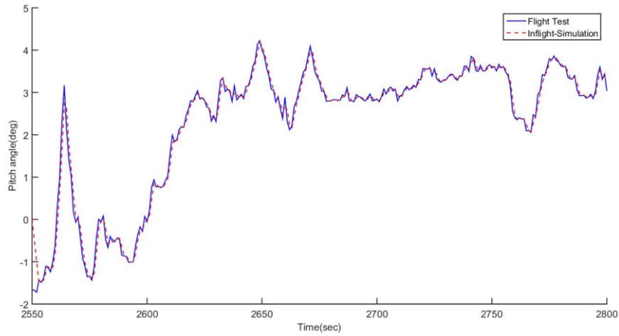
Fig. 18. The comparison of the pitch angle in the flight test of the guest aircraft vs. its in-flight simulation by the host aircraft simulator
