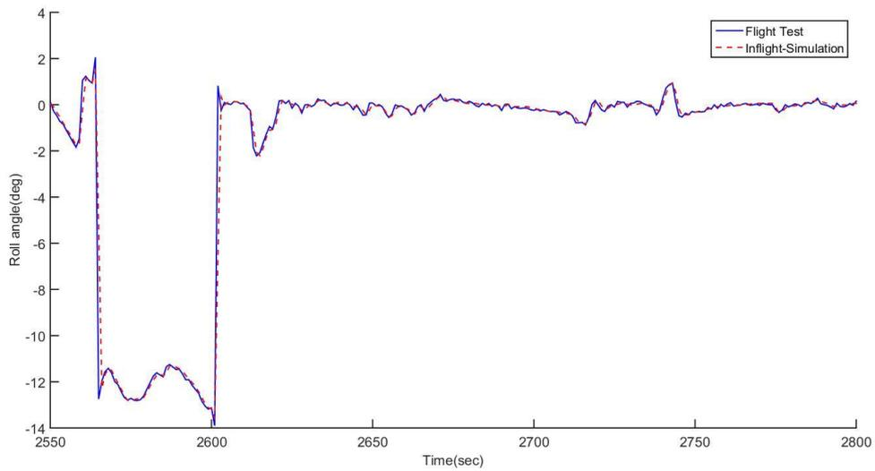
Fig. 19. The comparison of the roll angle in the flight test of the guest aircraft vs. its in-flight simulation by the host aircraft simulator
