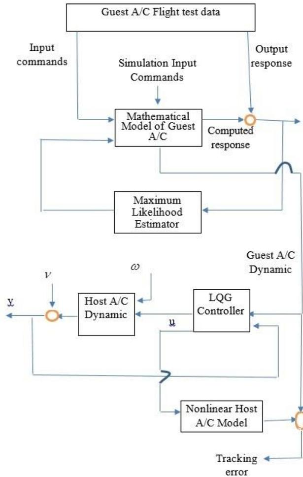
Fig. 9. The application concept of the LQG controller on the host aircraft simulator
