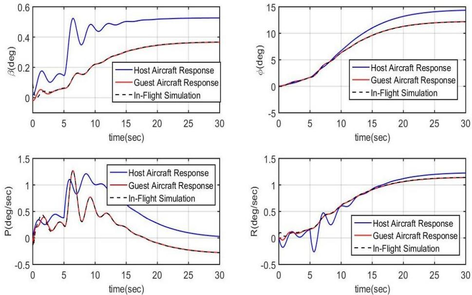
Fig. 14. a sample of nonlinear in-flight simulation of the guest aircraft response
