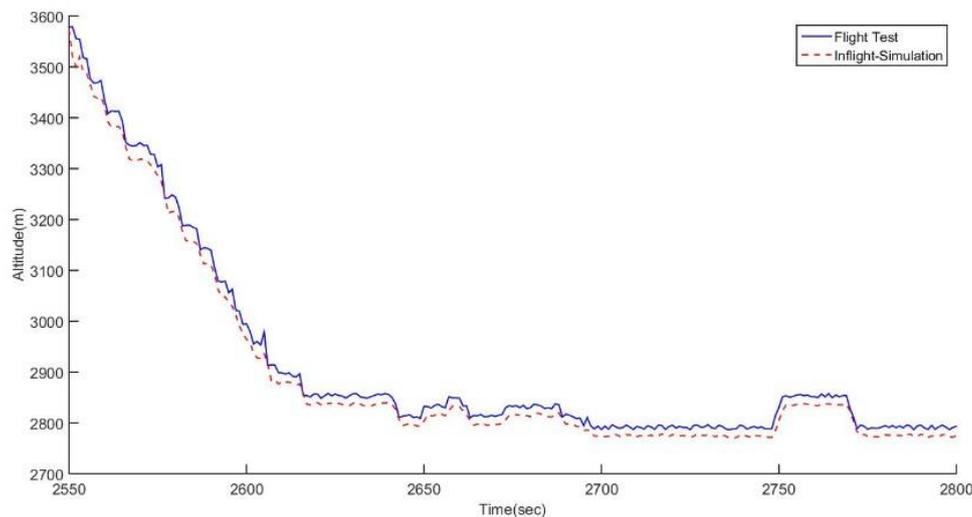
Fig. 17. The comparison of the aircraft altitude in the flight test of the guest aircraft vs. its in-flight simulation by the host aircraft simulator
