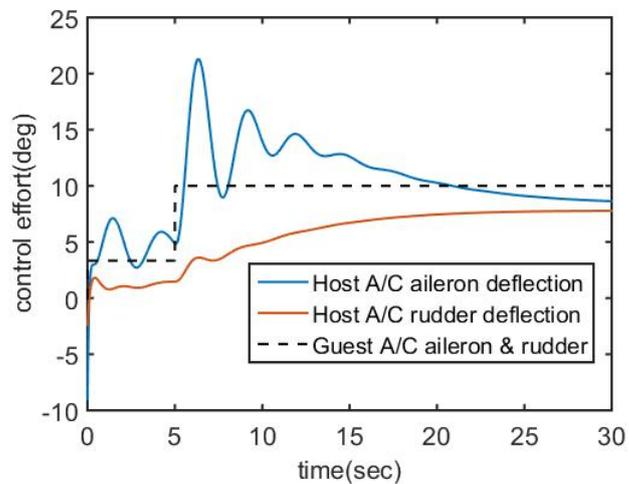
Fig. 13. A sample of aileron and rudder surface control input command for the of the guest aircraft against their equivalent control commands for the host aircraft
