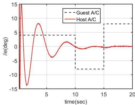
Fig. 10. A sample of elevator surface control input command for the guest aircraft against its equivalent control command for the host aircraft simulator
