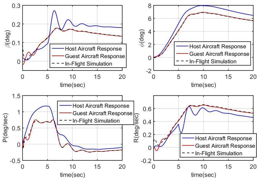
Fig. 8. A sample of linear in-flight simulation of the guest aircraft response in the lateral mode
