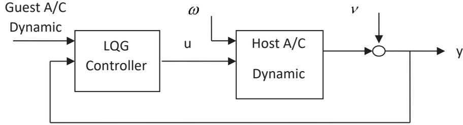
Fig. 6. The proper LQG controller for inflight simulation of the aircraft
