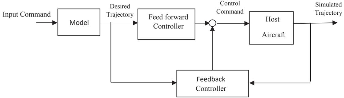
Fig. 1. A concept for the flight control system in an in-flight simulator
