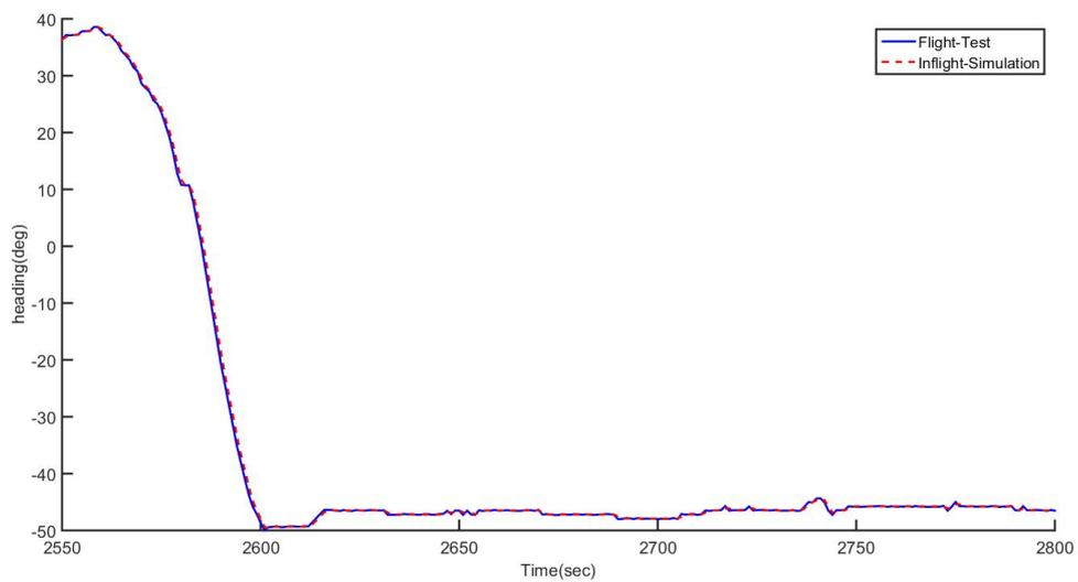
Fig. 20. The comparison of the heading in the flight test of the guest aircraft vs. its in-flight simulation by the host aircraft simulator
