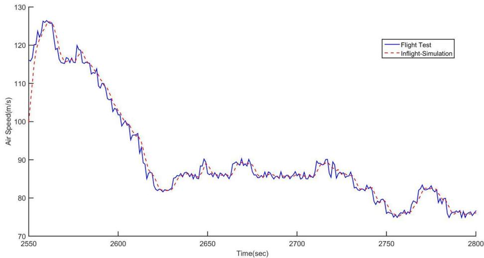
Fig. 16. The comparison of the airspeed flight test of the guest aircraft vs. its in-flight simulation by the host aircraft simulator
