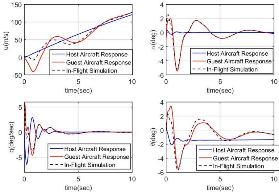
Fig. 7. A sample of linear in-flight simulation of the guest aircraft response in the longitudinal mode
