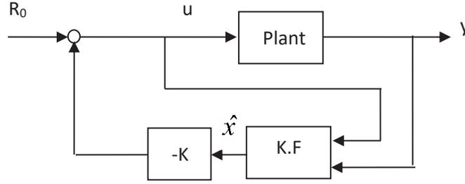
Fig. 3. The concept of the LQG controller [28]
