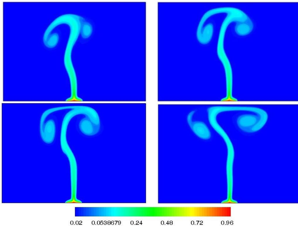
Fig. 8. Contaminat(Non-dimensional) concentration contours in the field without mass diffusion(left-top), with mass diffusion  $N = 0.4$ (right-top),  $N = 0.7$ (left-bottom) and  $N = 1.2$  (right-bottom) at  $t = 48s$ .
