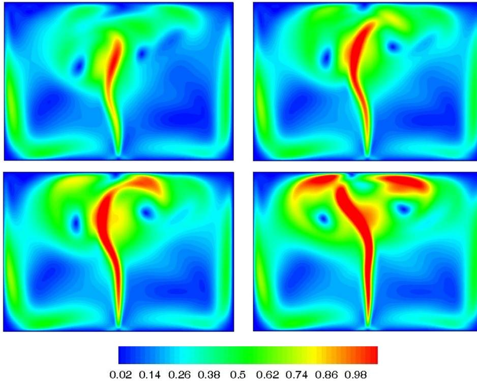
Fig. 7. Velocity magnitude(Non-dimensional) contours in the field without mass diffusion(left-top),with mass diffusion  $N = 0.4$ (right-top),  $N = 0.7$ (left-bottom) and  $N = 1.2$  (right-bottom) at  $t = 48s$ .
