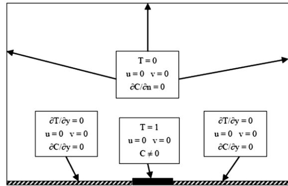
Fig. 1. The geometry of the computational domain and related boundary conditions.
