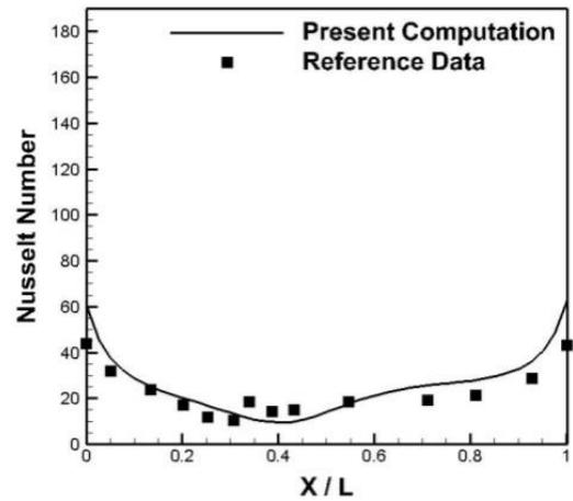
**Fig. 2. Distribution of local Nusselt number along horizontal heated plate compared experimental results[17], for conditions listed in Table 1.**
