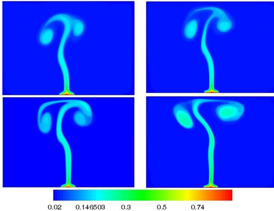
Fig. 3. Contours of temperature(Non-dimensional) in the field without mass diffusion(left),with mass diffusion  $N = 0.4$ (right-top),  $N = 0.7$ (left-bottom) and  $N = 1.2$  (right-bottom) at  $t = 48s$ .
