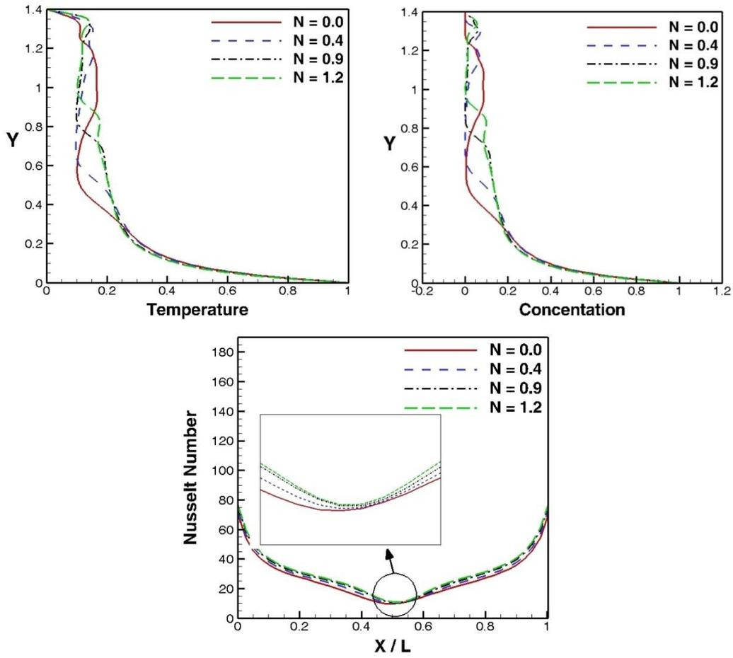
Fig. 5. Distribution of non-dimensional temperature (left) and concentration (right) along the horizontal center line and local Nusselt number along horizontal heated plate surface (bottom) at  $t = 48s$ , for different values of floatability number.
