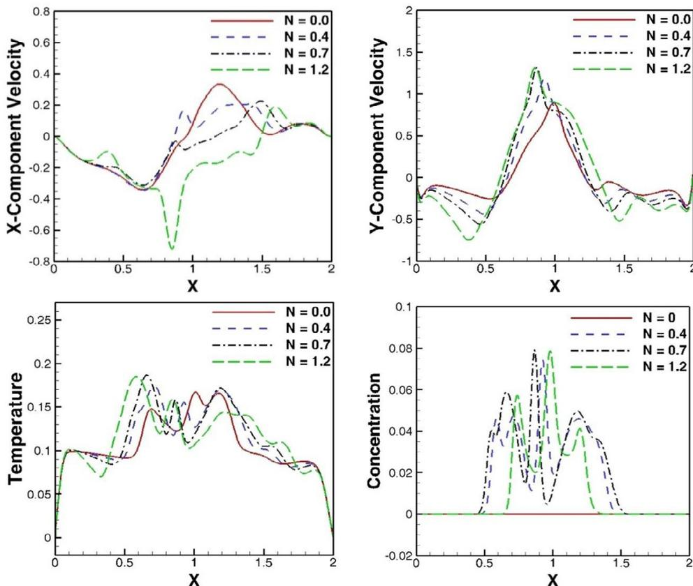
Fig. 4. Distribution of non-dimensional X-Component Velocity (top=left), Y-Component Velocity (top=right), Temperature (bottom-left) and Concentration(right-bottom) along horizontal line on  $y=1.048$ , at  $t = 48s$ , for different values of floatability number.
