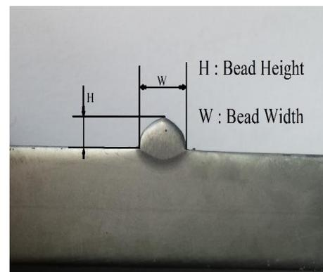
Fig. 3. The weld bead geometry on the etched part
