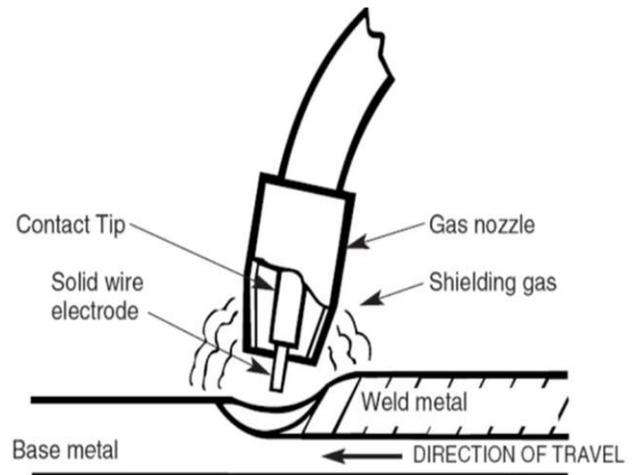
Fig. 1. Schematic diagram of Gas Metal Arc Welding
