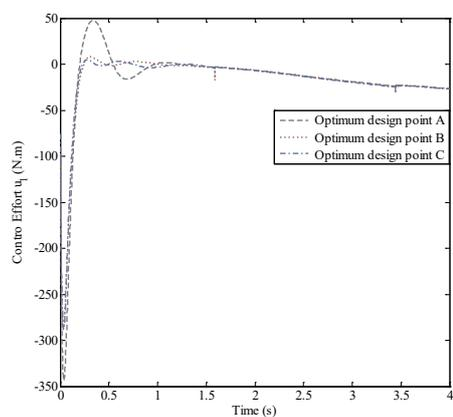
Fig. 6. Control effort  $u_1$  for the optimum design points A, B, and C shown in the Pareto front
