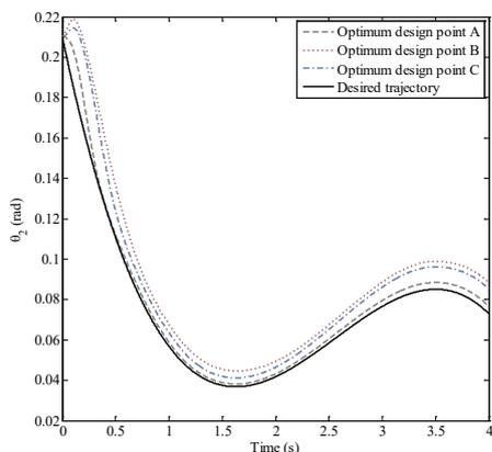
Fig. 4. Tracking trajectory  $\theta_2$  for the optimum design points A, B, and C shown in the Pareto front
