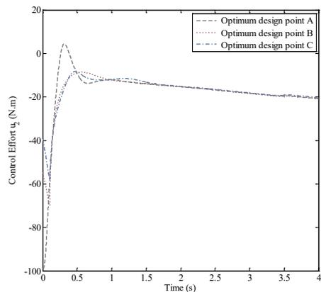
Fig. 7. Control effort  $u_2$  of the optimum design points A, B, and C shown in the Pareto front
