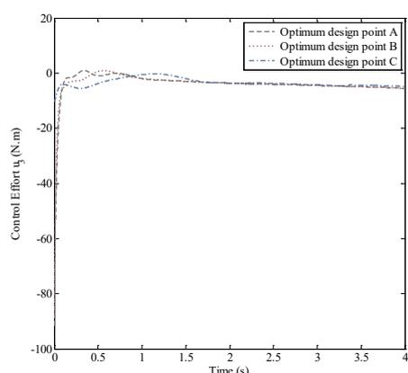
Fig. 8. Control effort  $u_3$  for the optimum design points A, B, and C shown in the Pareto front
