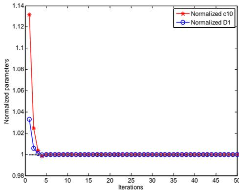
Figure3: convergence history of the normalized hyperelastic parameters.
