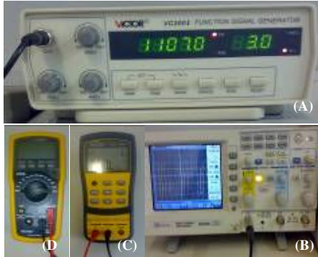
Figure 8: (A). Signal generator, (B). Oscilloscope, (C). LCR meter, (D). Multi-meter.
