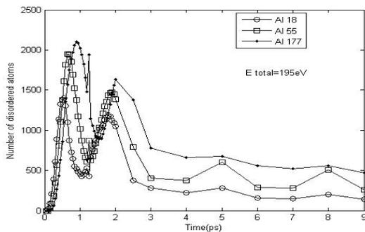
Figure 8. Time dependence of the number  $N_{dis}$  of disordered atoms in the substrate for  $E_T = 195eV$ .
