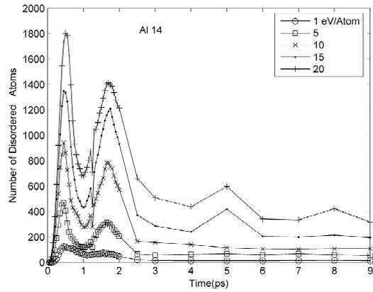
Figure 5. Time dependence of the number  $N_{dis}$  of disordered atoms in the substrate for  $Al_{47}$  and  $Al_{14}$ .
