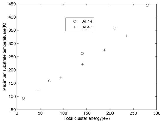
Figure 4. The maximum substrate temperature as a function of total energy.
