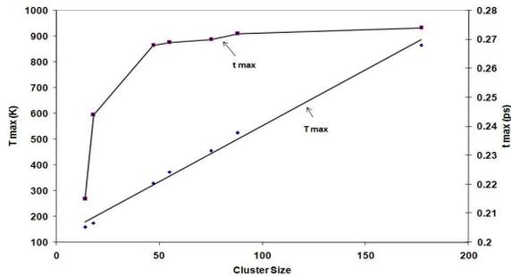
Figure 7. The temperature  $T_{max}$  and  $t_{max}$  as a function of cluster size in 5 eV/atom.
