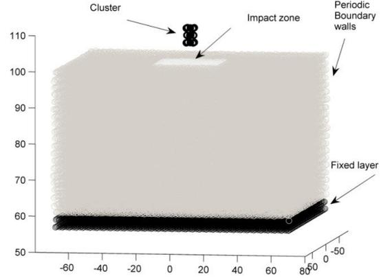
Figure1. The simulation system: Cluster; Impact zone; crystalline zone; fix zone.
