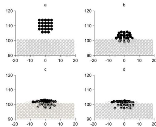
Figure2. Collision dynamics between an  $Al_{47}$  cluster with 1 eV/atom and an Al (100) substrate after 0 ps (a), 0.3 ps (b), 3 ps (c), 9 ps (d).
