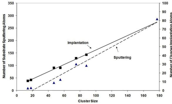
Figure 3. Number of implantation of atoms for all clusters in 5eV/atoms.
