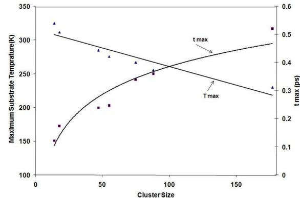
Figure 6. The temperature  $T_{max}$  and the time  $t_{max}$  for 195eV total energy as a function of cluster size.
