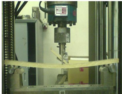
Fig.6. Three point bending test.
