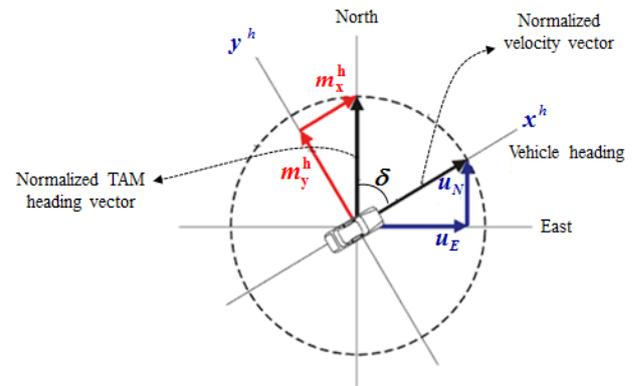
Fig. 3. TAM heading vector and normalized velocity vector
