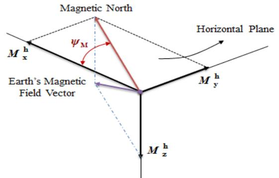
Fig. 1. Magnetic heading angle and horizontal plane components of the magnetic field vector
