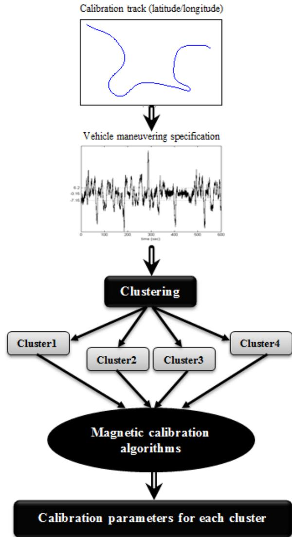
Fig. 4. Schematic view of the proposed clustering calibration method
