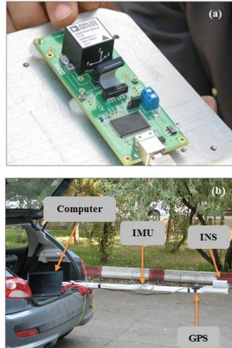
Fig. 5. (a) IMU-ADIS16407, (b) Experiment devices placed on the vehicle
