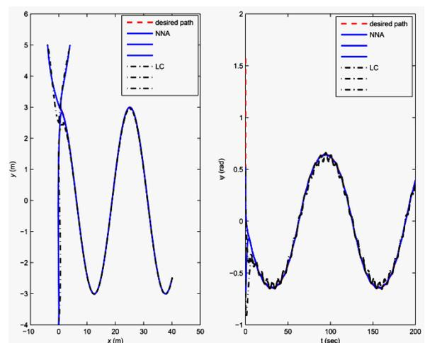
Fig. 6. Left: trajectories in horizontal plane. Right: curve of heading ASVs
