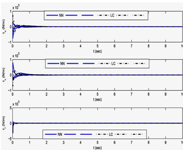
Fig. 8. Control inputs of ASVs during consensus tracking
