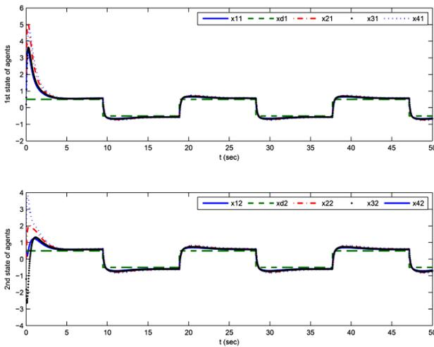
Fig. 2. Desired signal tracking by the states of the agents
