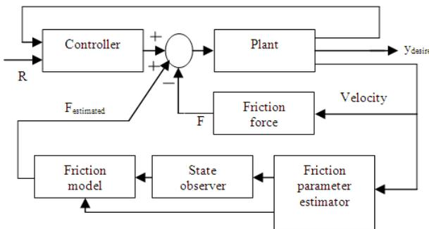
Fig. 9. General procedure for friction compensation [1].
