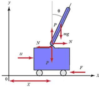
Fig. 1. Schematic of SIPC system with exerted forces on it [1].
