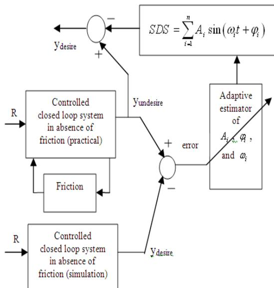
Fig. 10. Overall scheme of proposed adaptive friction compensator technique [1].
