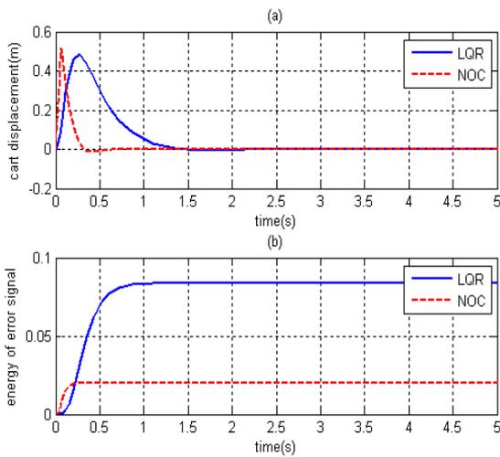
**Fig. 5. Performance of NOC on cart position in closed loop system in comparison with LQR. (a): cart position, (b): energy of error signal.**
