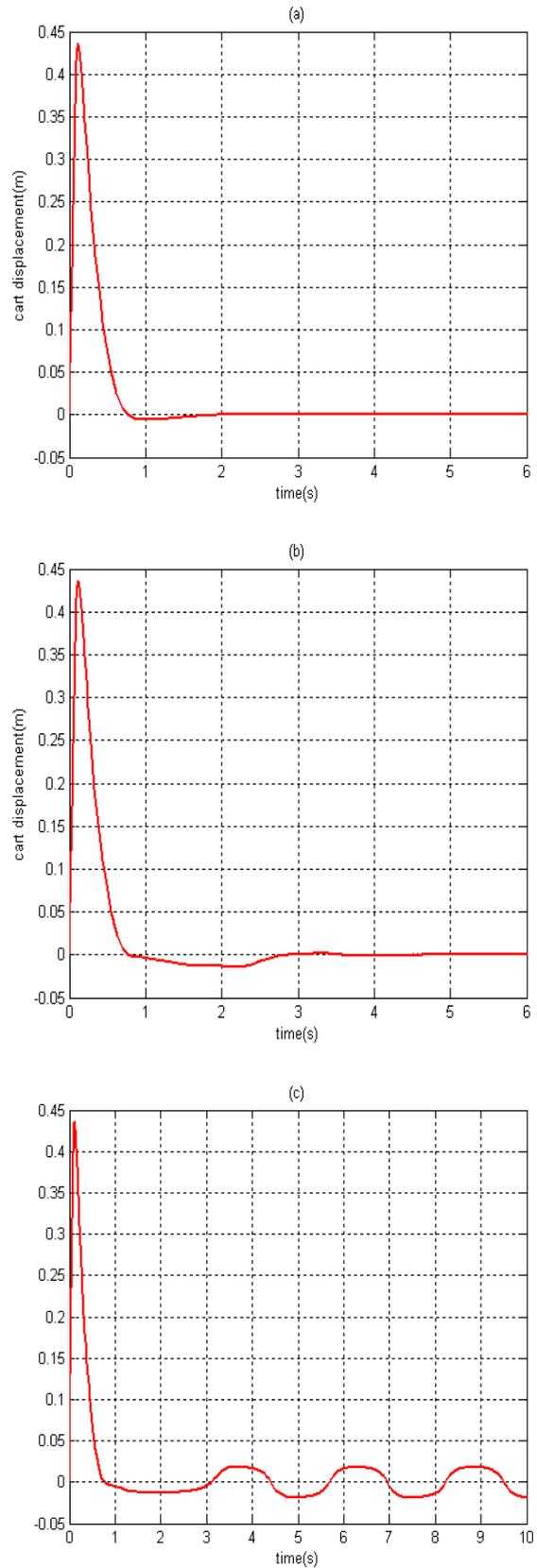
**Fig. 7. . Capability of NOC in encountering with different models of friction. (a): static model, (b): exponential mode, (c): LuGre dynamic model. System is actuated by initial conditions**
