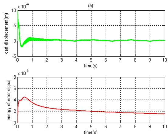
Fig. 13. (a): cart modified position response to initial condition  $x_0^T = [0 \ 0.3488 \ 0 \ 0]$  in presence of friction compensation loop and nonlinear optimal controller, (b): energy of error signal
