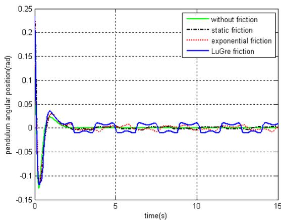
Fig. 4. Pendulum angular displacement response to initial condition  $x_0^T = [0 \ 0.2325 \ 0 \ 0]$  in closed loop system.
