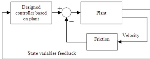
Fig. 2. Structure of closed loop system in presence of friction [1].
