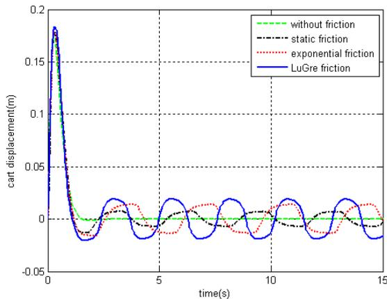
Fig. 3. Cart displacement response to initial condition  $x_0^T = [0 \ 0.2325 \ 0 \ 0]$  in closed loop system.
