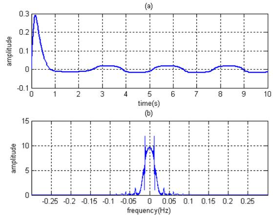
Fig. 11. (a): Noise signal which is difference between response of cart displacement in presence and absence of friction to initial condition  $x_0^T = [0 \ 0.3488 \ 0 \ 0]$ , (b): Frequency spectrum of noise signal.
