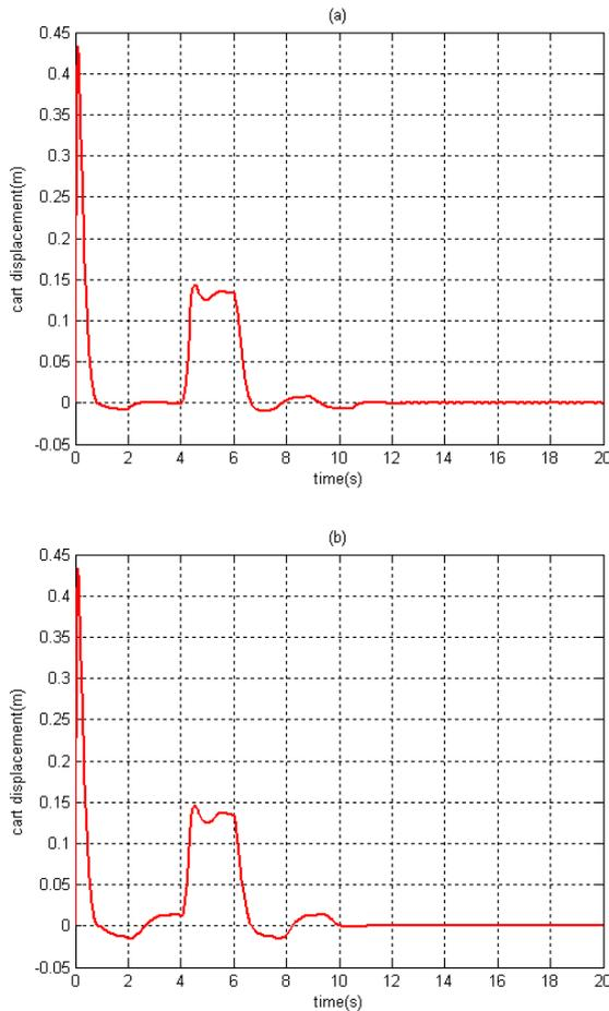
Fig. 8 . Response of cart position in closed loop system in presence of friction with uncertainty for cart mass (20 percent) and pendulum mass (10 percent) and exerted disturbance signal, (a): static model,(b): exponential model.
