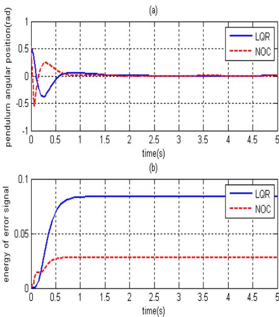
**Fig. 6. Performance of NOC on pendulum angular position in closed loop system in comparison with LQR. (a): pendulum angular position, (b): energy of error signal**
