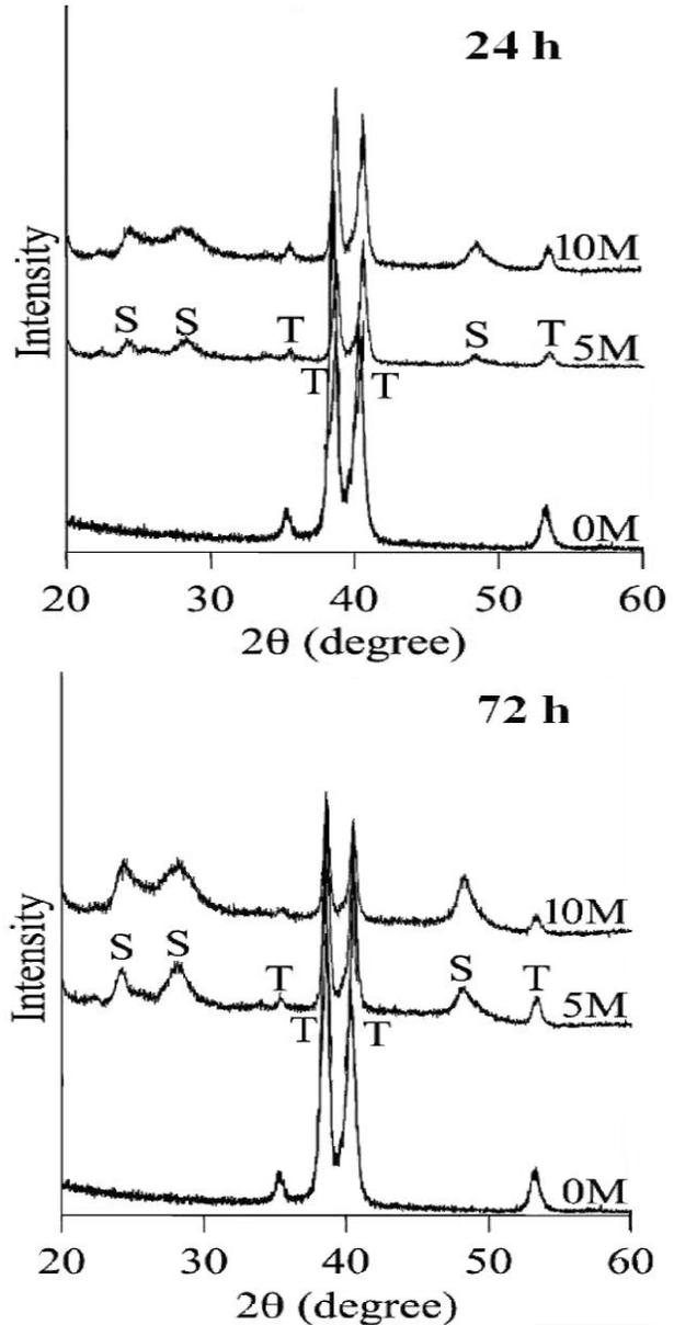
Figure 1: TF-XRD patterns of the specimens subjected to 0, 5, 10 M NaOH treatment at 60 °C for 24h, 72h. T: titanium and S: sodium titanate.
