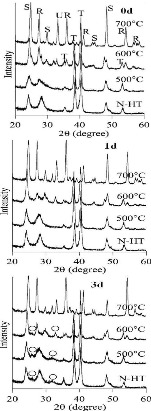
Figure 5: TF-XRD patterns of the specimens subjected to 5 M NaOH treatment at 80 °C for 72 h without heat treatment (N-HT) or heat-treated at 500, 600 or 700 °C for 1 h, and soaked in SBF for 0, 1, 2 or 3 days, R: rutile, T: titanium, S: so sodium titanate, O: apatite, and U: unknown.
