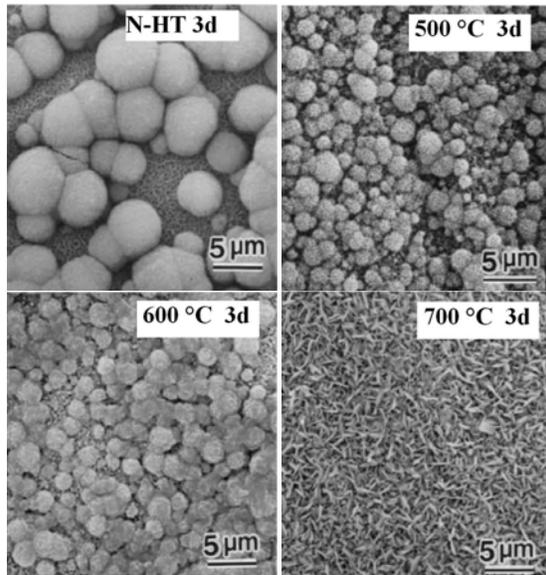
Figure 7: Surface morphologies (by SEM) of the specimens subjected to 5 M NaOH treatment, without heat treatment (N-HT) or heat-treated at 500, 600 or 700 °C for 1 h, and soaked in SBF for 3 days.
