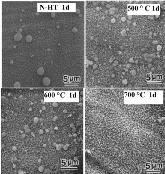
Figure 6: Surface morphologies (by SEM) of the specimens subjected to 5 M NaOH treatment, without heat treatment (N-HT) or heat-treated at 500, 600 or 700 °C for 1 h, and soaked in SBF for 1 days.
