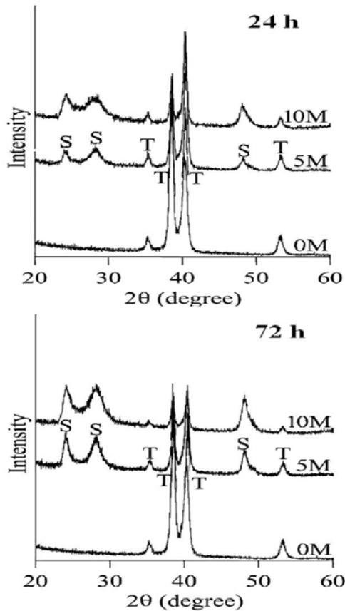
Figure 2: TF-XRD patterns of the specimens subjected to 0, 5, 10 M NaOH treatment at 80 °C for 24h, 72h. T: titanium and S: sodium titanate.
