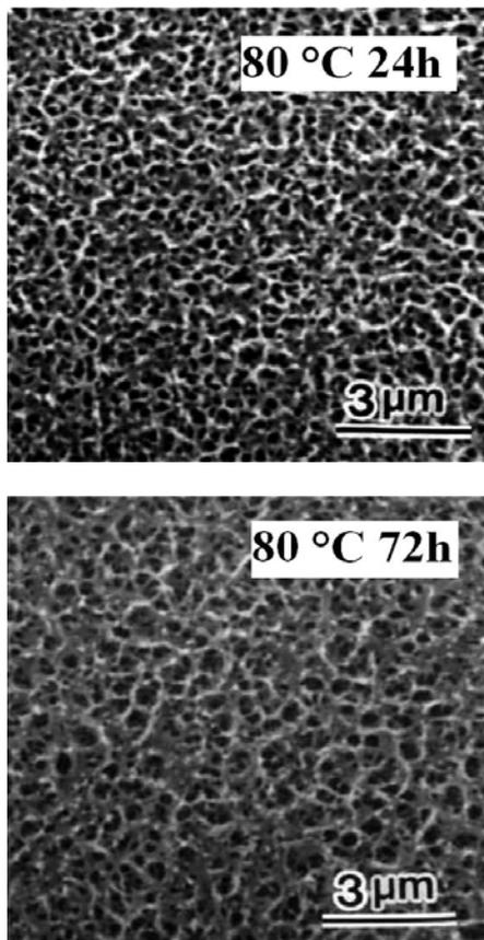
Figure 4: Surface morphologies (by SEM) of the specimens subjected to 5 M NaOH treatment at either 60 or 80 °C for 24, 72 h.
