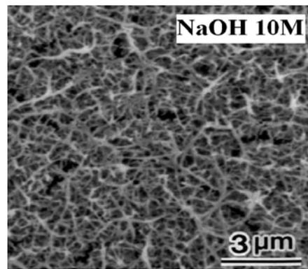
Figure 3: Surface morphologies (by SEM) of the specimens subjected to 0, 5, 10 M NaOH treatment at 60 °C for 72h.
