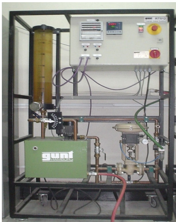
Figure 11: Level control process.
