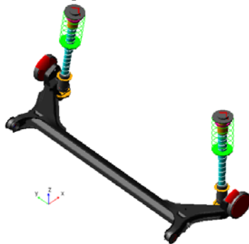
Figure 4: Rear suspension model in ADAMS.
