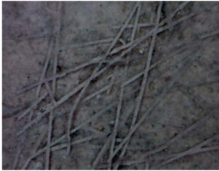
Figure 16: Aggregation of PAN fibers on matrix surface.
