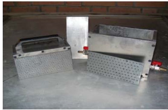
Figure 5: Parts of specimen production equipment.
